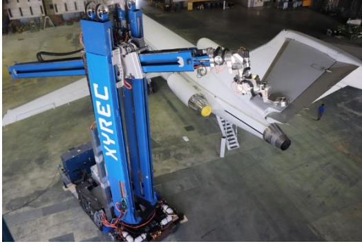
Testing of the new de-painting technology is conducted on a B727-200 aircraft.
