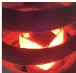
Building blocks for extra-terrestrial colonization: Powdered basaltic matter is subjected to high temperatures in the research team's experimental vacuum oven and then molded into bricks to create building components for landing pads on the Moon and Mars. Image credit: Astroport Space Technologies/WEX Foundation.
