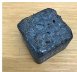
Building blocks for extra-terrestrial colonization: Powdered basaltic matter is subjected to high temperatures in the research team's experimental vacuum oven and then molded into bricks to create building components for landing pads on the Moon and Mars. Image credit: Astroport Space Technologies/WEX Foundation.
