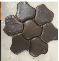
Building blocks for extra-terrestrial colonization: Powdered basaltic matter is subjected to high temperatures in the research team's experimental vacuum oven and then molded into bricks to create building components for landing pads on the Moon and Mars. Image credit: Astroport Space Technologies/WEX Foundation.
