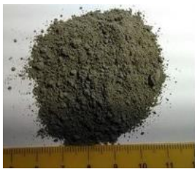
Building blocks for extra-terrestrial colonization: Powdered basaltic matter is subjected to high temperatures in the research team's experimental vacuum oven and then molded into bricks to create building components for landing pads on the Moon and Mars. Image credit: Astroport Space Technologies/WEX Foundation.
