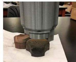
Building blocks for extra-terrestrial colonization: Powdered basaltic matter is subjected to high temperatures in the research team's experimental vacuum oven and then molded into bricks to create building components for landing pads on the Moon and Mars. Image credit: Astroport Space Technologies/WEX Foundation.
