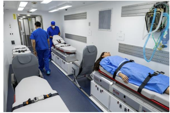
Interior image of Knight Aerospace's second completed medical module, which can provide a full spectrum of hospital grade care while in flight or as a standalone emergency medical facility on the ground.
