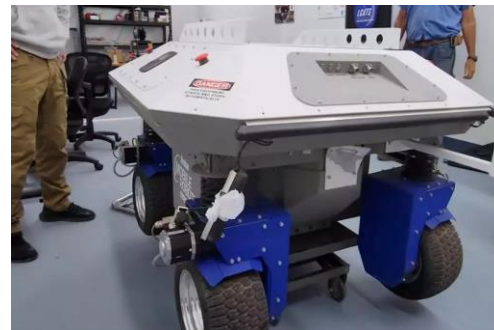
The Brickbot is a proof-of-concept project to show that regolith bricks can be made on the moon. Astroport Space Technologies officials are targeting 2026 for delivering this test vehicle to the lunar surface.
